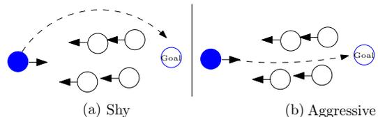
Figure 3: Example of ORCA behaviors. (a) Using a shy model,  $\alpha$  decides to move around the group. (b) Using the aggressive model, instead,  $\alpha$  makes way between the incoming agents to reach the goal faster.
