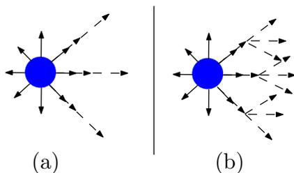
Figure 2: The 9 actions of *VelPlan* correspond to moving at 1.5 m/s with different angles with respect to the goal:  $0^\circ$ ,  $\beta$ ,  $-\beta$ ,  $90^\circ$ ,  $-90^\circ$ ,  $180^\circ$ ,  $180^\circ + \beta$ ,  $180^\circ - \beta$  and complete stop. We use  $\beta = 45^\circ$ . (a) Simple plans consist of single actions for the entire time horizon. (b) More complex plans are computed if planning time allows.
